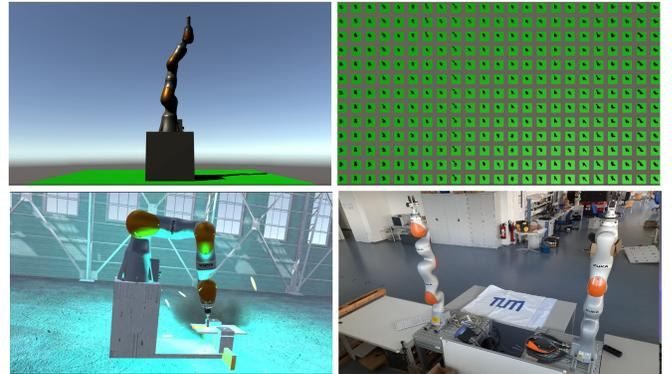
Fig. 2. The simulation platform and the real robots. Upper left: Simple simulation environment for a reaching task. Upper right: Top-down view of matrix of simulation environments running in parallel. Bottom Left: Simulation of highly-realistic rendering and physics. Bottom right: The Kuka<sup>TM</sup> iiwa manipulators [18] used in the experiments.
